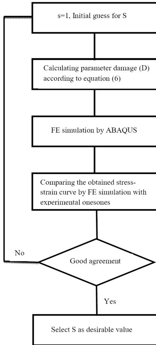
**Fig.2.** Flowchart for picking the damage model constants ( $s$  and  $S$ ).
