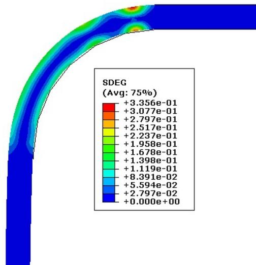
Fig.7. scalar stiffness degradation distribution
