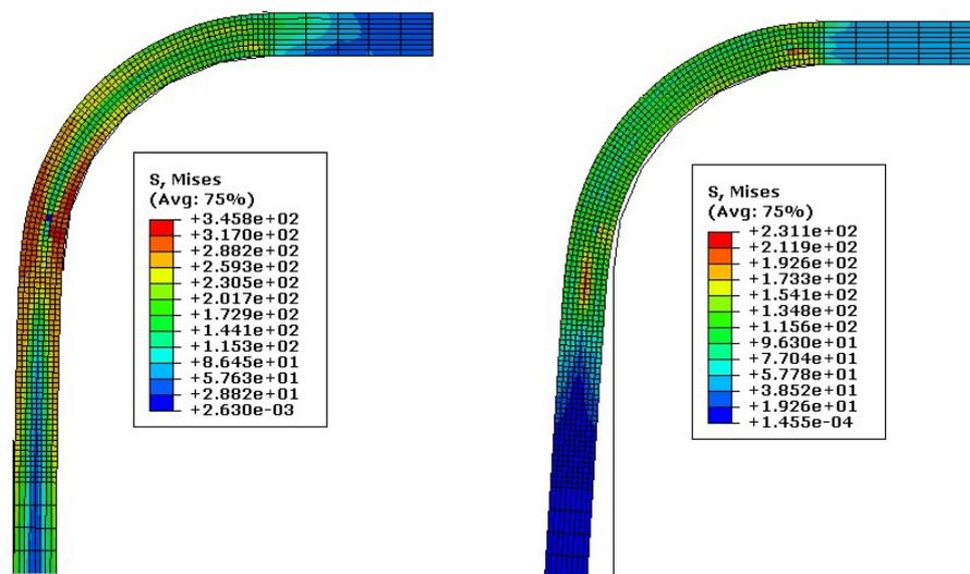
**Fig.5.** Distribution of von Mises stress in the blank (left: loading, right: springback)
