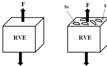
Fig.1. one-dimensional element (Left: no damage, Right: damaged)
