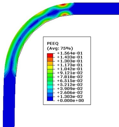
**Fig.6.** Equivalent plastic strain distribution
