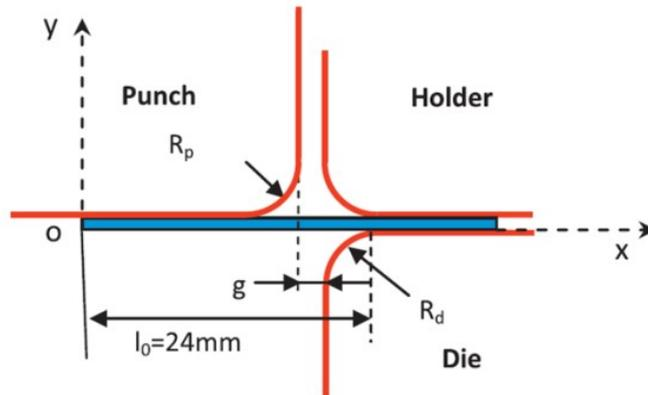
Fig. 4. Schematic illustration of L-bending test [7].
