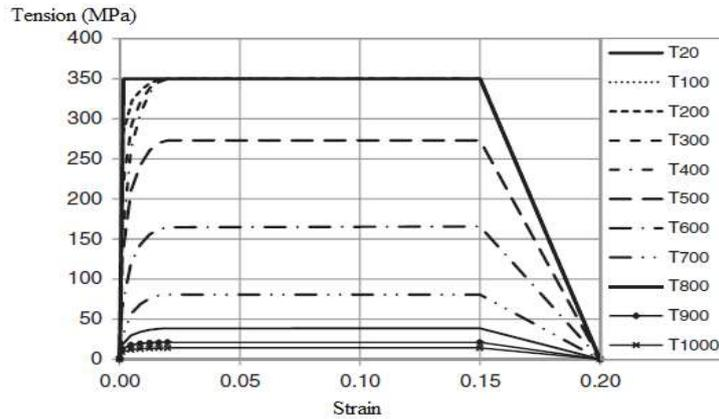
Fig. 2. Stress-strain curve of the steel affected by increasing the temperature [11]
