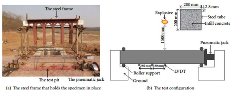
Fig. 1. Test setup (Zhang et al. [9])
