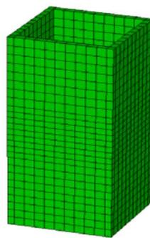
**Fig. 5.** Finite element model of the steel wall in concrete-filled steel columns
