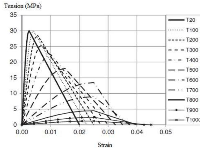
Fig. 3. Stress-strain curve of the concrete affected by increasing the temperature [12]
