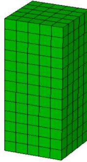
**Fig. 6.** Finite element model of the concrete core in concrete-filled steel columns
