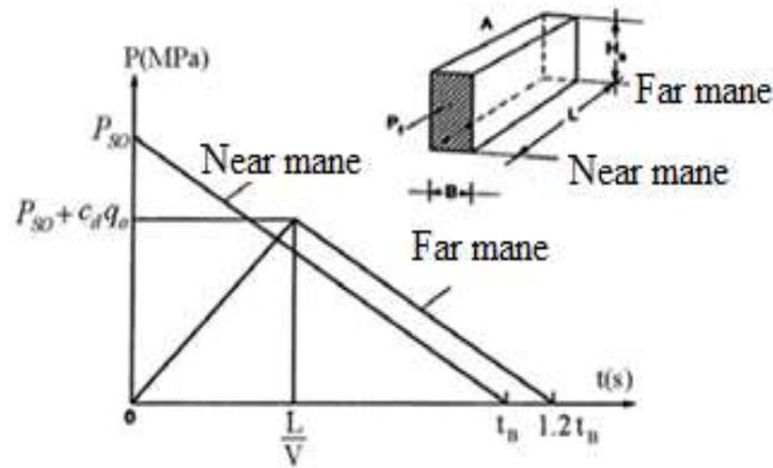
Fig. 9. Pressure changes on the side faces and the roof of the structure
