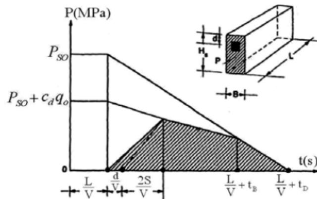
Fig. 10. Pressure changes on the behind face of the structure
