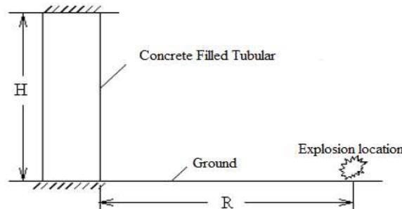
**Fig. 4.** Concrete-filled steel column under the blast load
