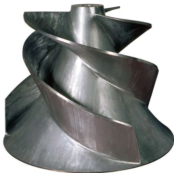
Fig.3. Manufactured fish-friendly turbine with three blades [14]
