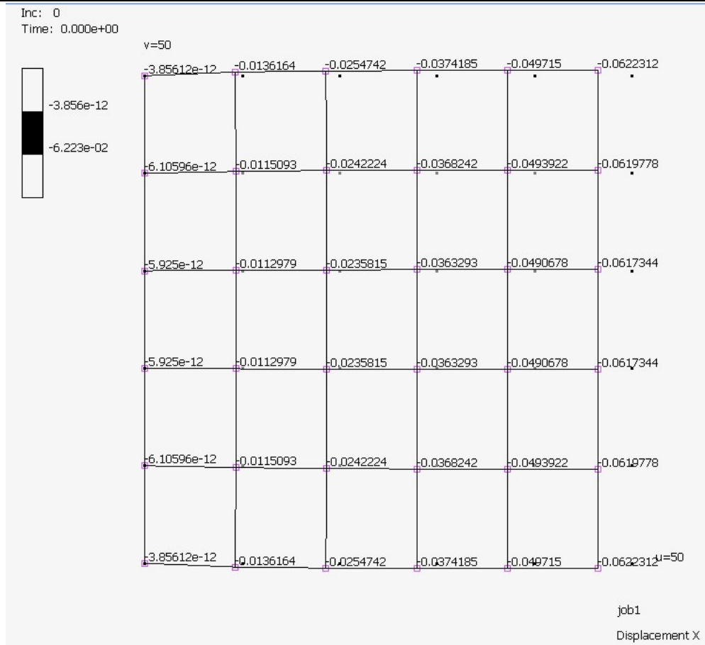
Fig. A.2. The nodal X-displacement performing FEA using MSc Marc®
