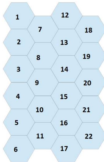
Fig. 7. The six-node hexagonal mesh with the element numbers inside
