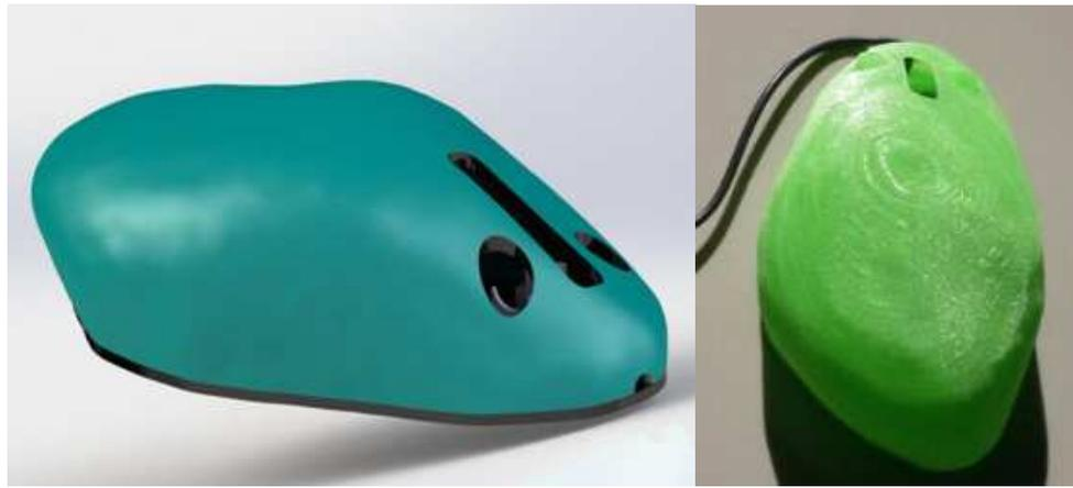
Fig. 3. Designing and the prototyped right-handed mouse
