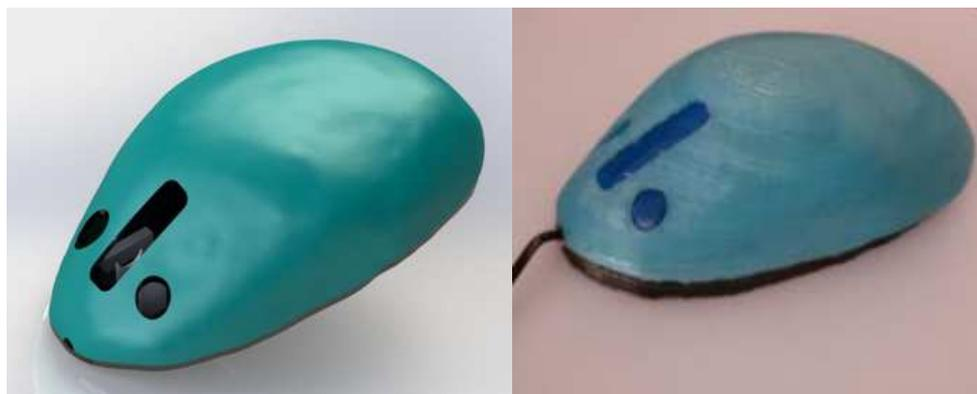
Fig. 2. Designing and the prototyped left-handed mouse
