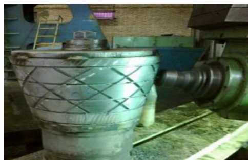
Fig. 5. Metallic mandrel for composite lattice truncated cone
