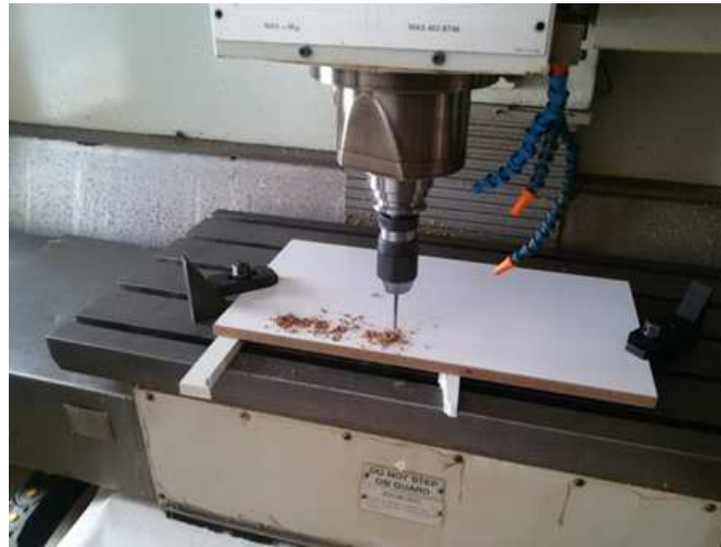
Fig. 1. The drilling process of the MDF panel on a vertical machining centre.
