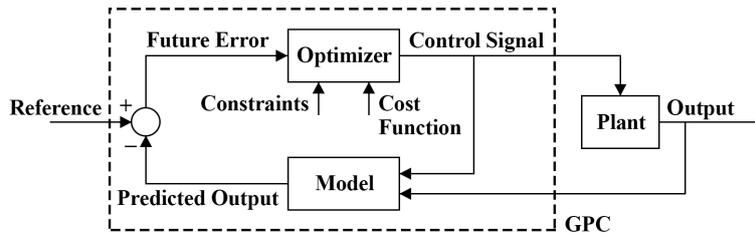
Fig. 6. GPC Controller Structure
