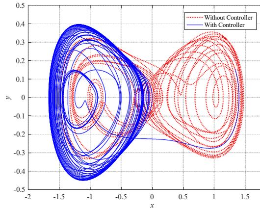
Fig. 11. Phase plane with  $f_e = 30$  , after applying GPC control input
