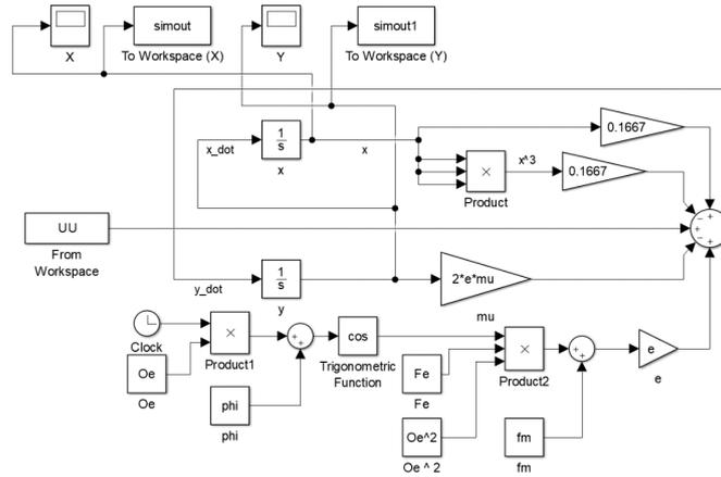
Fig. 7. Gear transmission system in MATLAB Simulink
