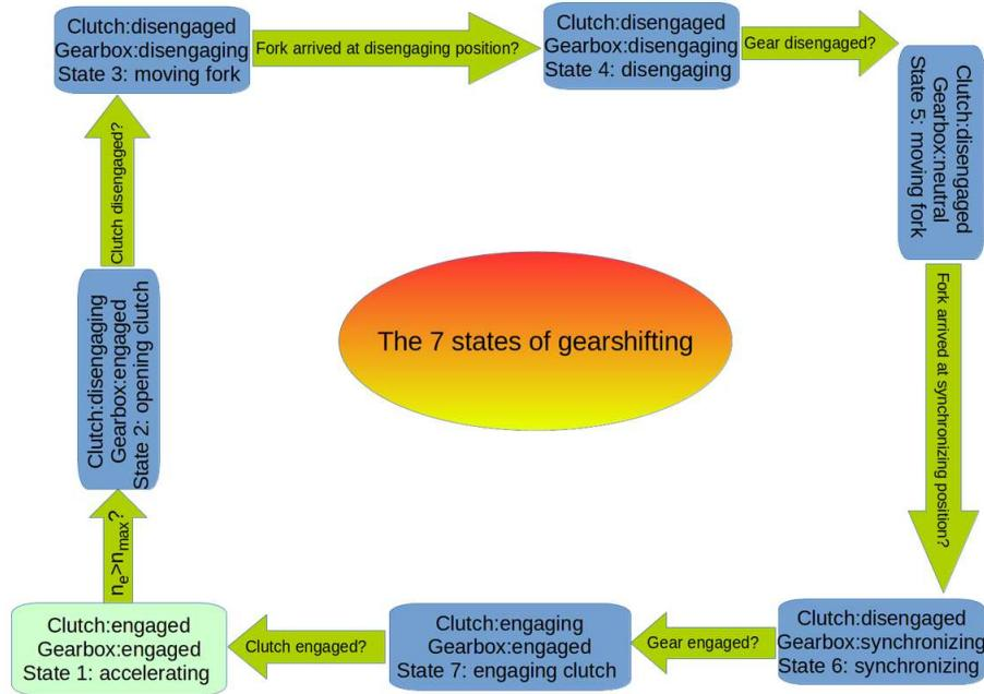
Fig. 7. The gearshifting procedure and the involved state changes.
