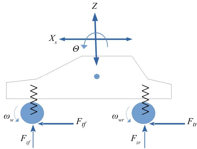
Fig. 4. The longitudinal model of the vehicle.
