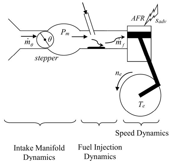
Fig. 1. The engine subsystems.
