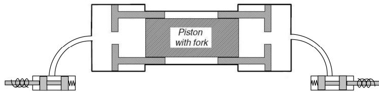
Fig. 3. An automated gearbox which has two distinct electrohydraulic actuators for moving the fork from one side to the other.
