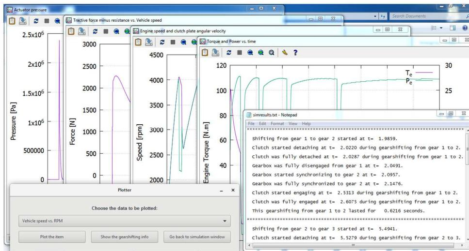
Fig. 6. The capability of Powertrain Simulator in plotting and extracting gearshifting details.
