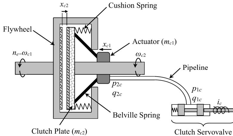
Fig. 2. The clutch system includes the servovalve, piping and the actuator along with the mechanical parts.
