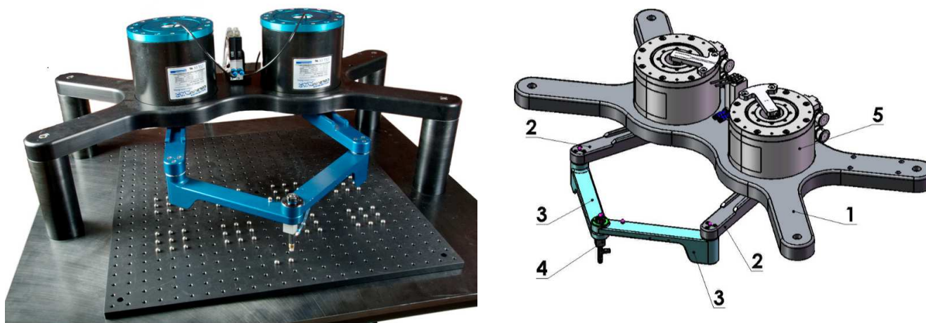
Fig. 1. Photo of DexTAR robot and its schematic configuration presented in [28]: real model (left) and virtual prototype: 1 - the base plate; 2 - the first set of rods; 3 - the second set of rods; 4 - end effector; 5 - servo motors,
