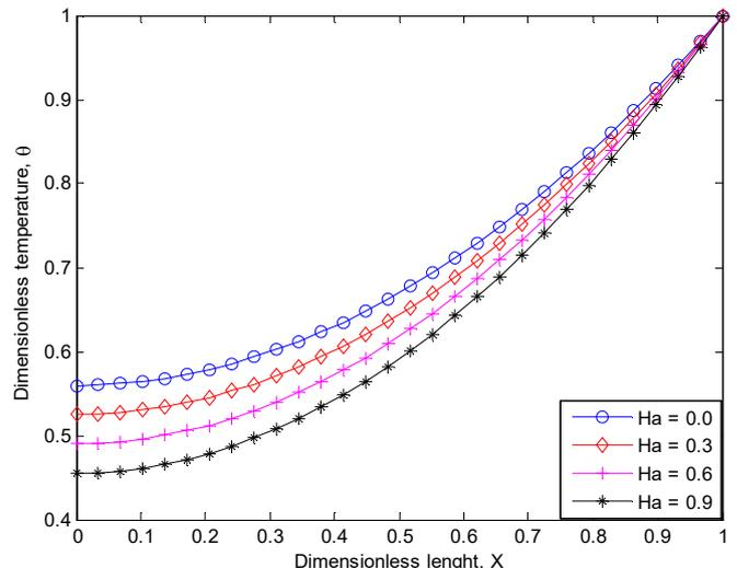
Fig. 5. Effects of Hartmann number on the nondimensional temperature distribution in the fin
