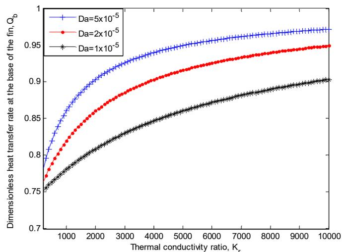
Fig. 9. Effects of Darcy number on the rate of heat transfer
