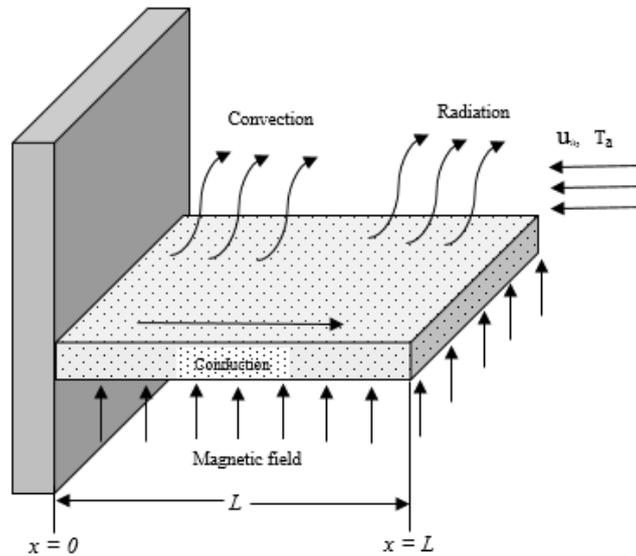
Fig. 1. Schematic configuration of the convective-radiative longitudinal porous fin subjected to magnetic field
