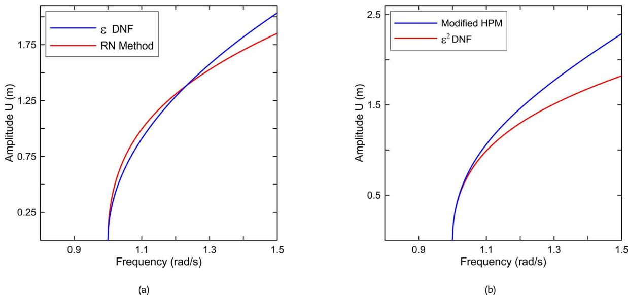
Fig. 2. Comparison between DNF results and other methods for the cubic-quintic oscillator: (a)  $\varepsilon$ -order DNF and the method of Renormalization (RN method), (b)  $\varepsilon^2$ -order DNF and the modified homotopy method (Modified HPM). Parameter values are:  $\omega_n = 1$  rad/s,  $\alpha_1 = 0.2$  and  $\alpha_2 = 0.1$ .
