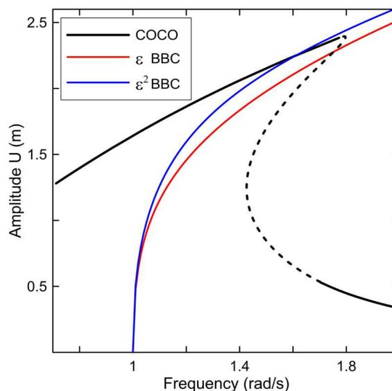
**Fig. 5.** Comparison of DNF results and COCO results for the nonlinear oscillator in Eq. (23), the solid blue and red curves represent the analytical DNF results for  $\varepsilon$  and  $\varepsilon^2$  accuracies, respectively. Moreover, the black line denotes the frequency-response curve computed using COCO; the solid black line shows the stable region of the response while the dashed black line represents the unstable region.
