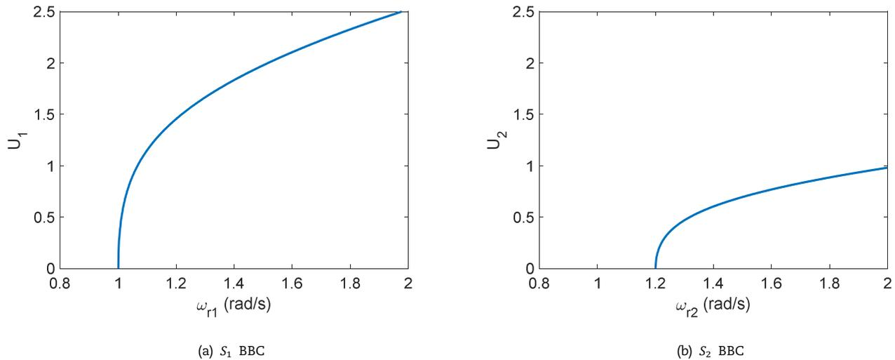
Fig. 7. Single-mode backbone curves of the 2-DOF oscillator studied in Section 5: (a)  $S_1$  backbone curve which represents the projection of  $U_1$  against  $\omega_{r1}$ , (b)  $S_2$  backbone curve which represents the projection of  $U_2$  against  $\omega_{r2}$ . Parameter values are:  $\omega_{n1} = 1$  rad/s,  $\omega_{n2} = 1.2$  rad/s and  $\kappa_{3,1} = \kappa_{3,2} = \kappa_{5,1} = \kappa_{5,2} = 0.1$ .
