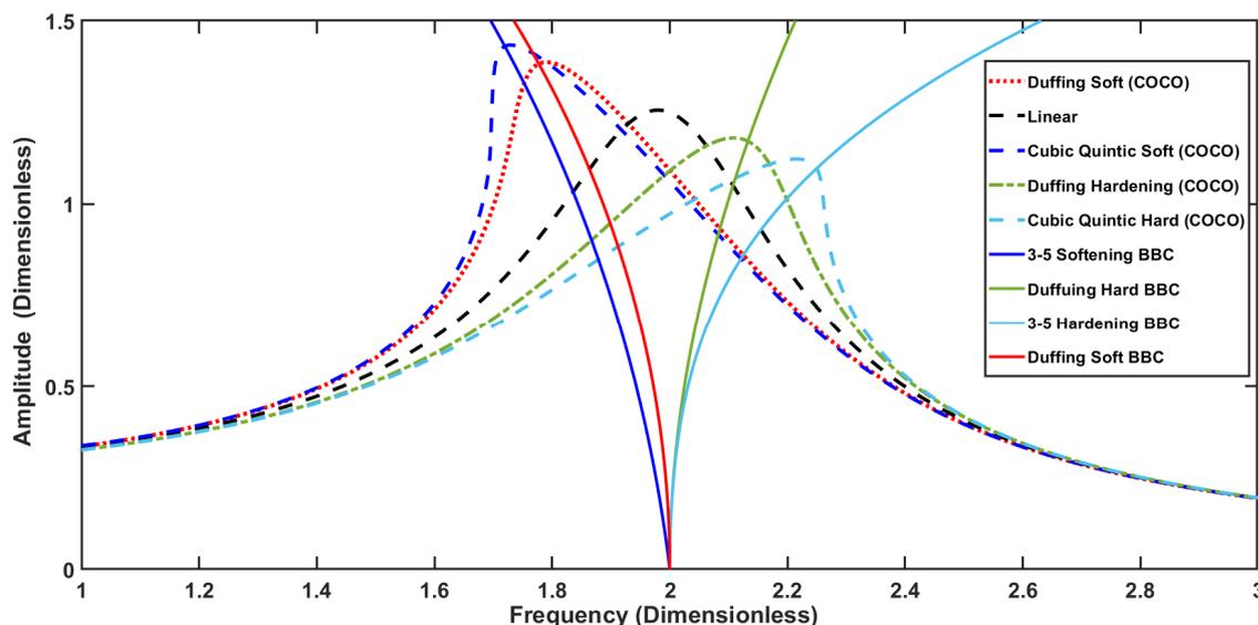
**Fig. 4.** Backbone curves and forced frequency response functions for different values of the nonlinear coefficients; solid lines represent backbone curves and dashed lines show the locus of the maximum displacement amplitude of the equivalent period orbit with forcing and damping added. Parameter values are:  $\omega_n = 2$  rad/s, and  $\alpha_1 = \alpha_2 = 0.1$  for the hardening cases, and  $\alpha_1 = \alpha_2 = -0.1$  for the softening cases.
