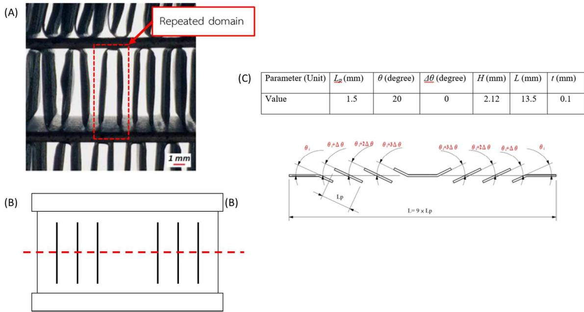
Fig. 1. Geometric parameter of a louver fin from Jang and Chen [13].
