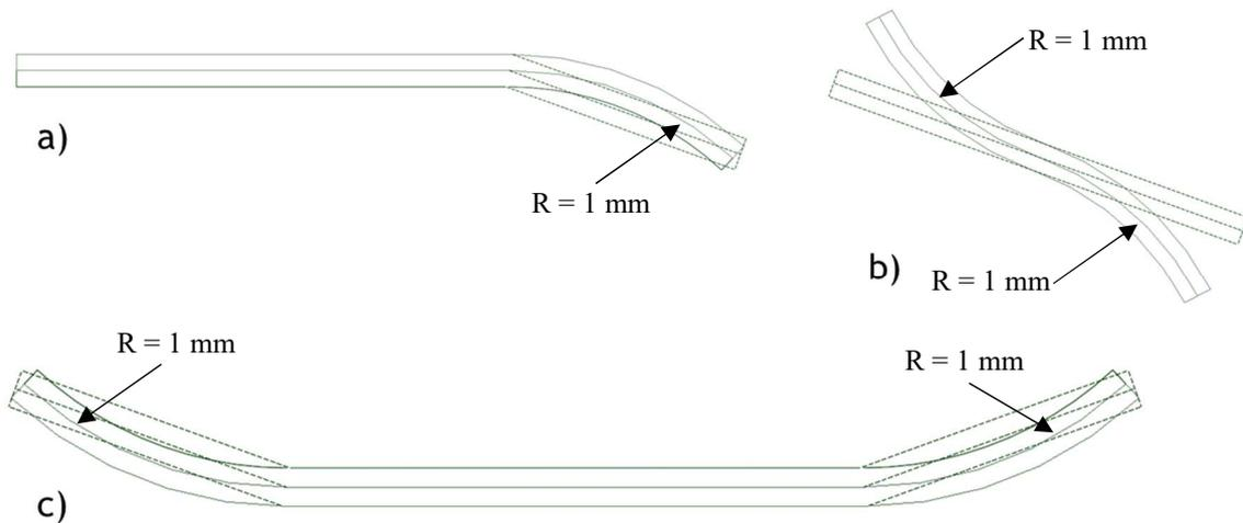
Fig. 3. Curved fin (solid line) interfered with the ordinary flat fin (dash line) at (a) the first (Fin 1) and last (Fin 7) fins, (b) the second (Fin 2), third (Fin 3), fifth (Fin 5), and sixth fins (Fin 6) and (c) the fourth fin (Fin 4).
