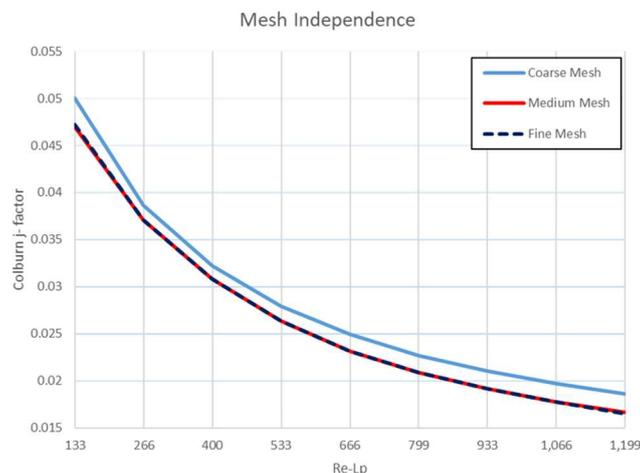
**Fig. 7.** Mesh independence by comparing Colburn  $j$ -factor among three mesh setting—the blue and red solid lines represent the coarse and medium mesh, respectively, and dashed line represents the fine mesh.
