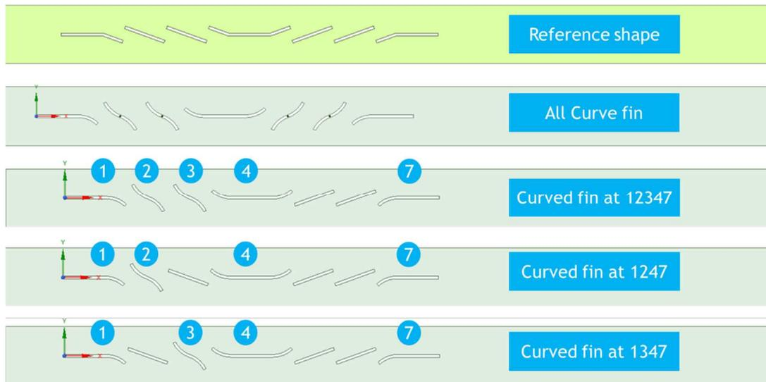
Fig. 2. Five designs labeled using the location of the curved fins.
