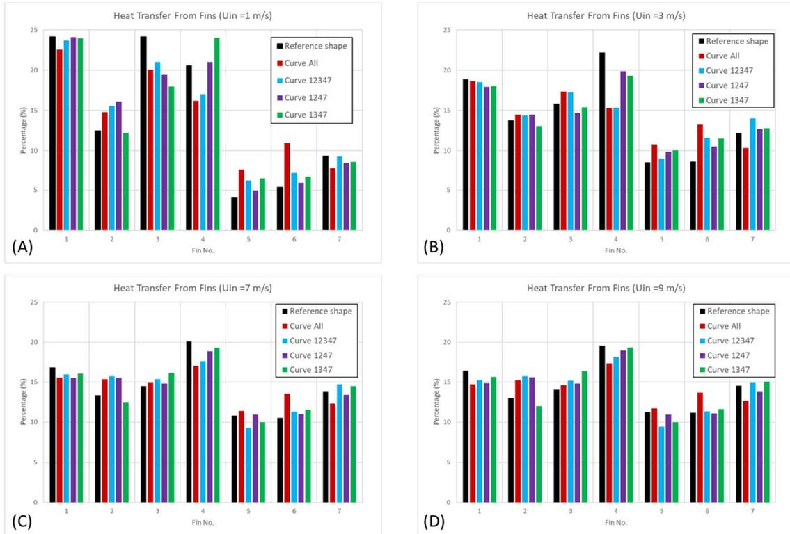
Fig. 11. Amount of heat transfer from fin to airflow at various inlet velocities; (A) 1 m/s, (B) 3 m/s, (C) 7 m/s, and (D) 9 m/s.
