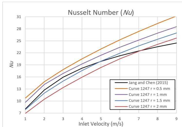
Fig. 12. Variation of curved fin radius in case of 1247.
