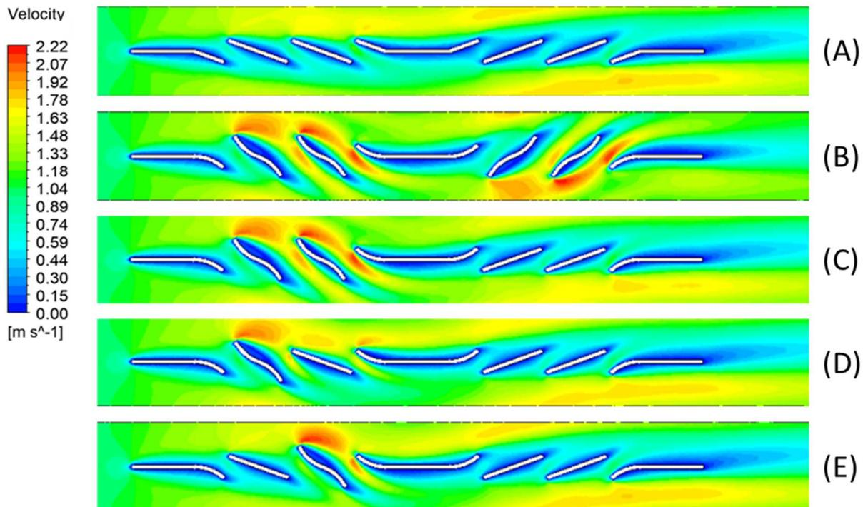
Fig. 8. Velocity contour of different shapes at an inlet velocity of 1 m/s.
