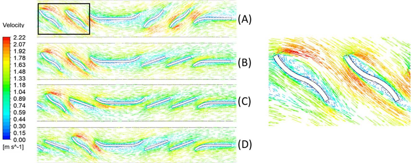
Fig. 9. Vector plot of different shapes at an inlet velocity of 1 m/s with circles indicating the locations of vortices with black circles in the case of (A) All curved, (B) Curve 12347, (C) Curve 1247, and (D) Curve 1347.
