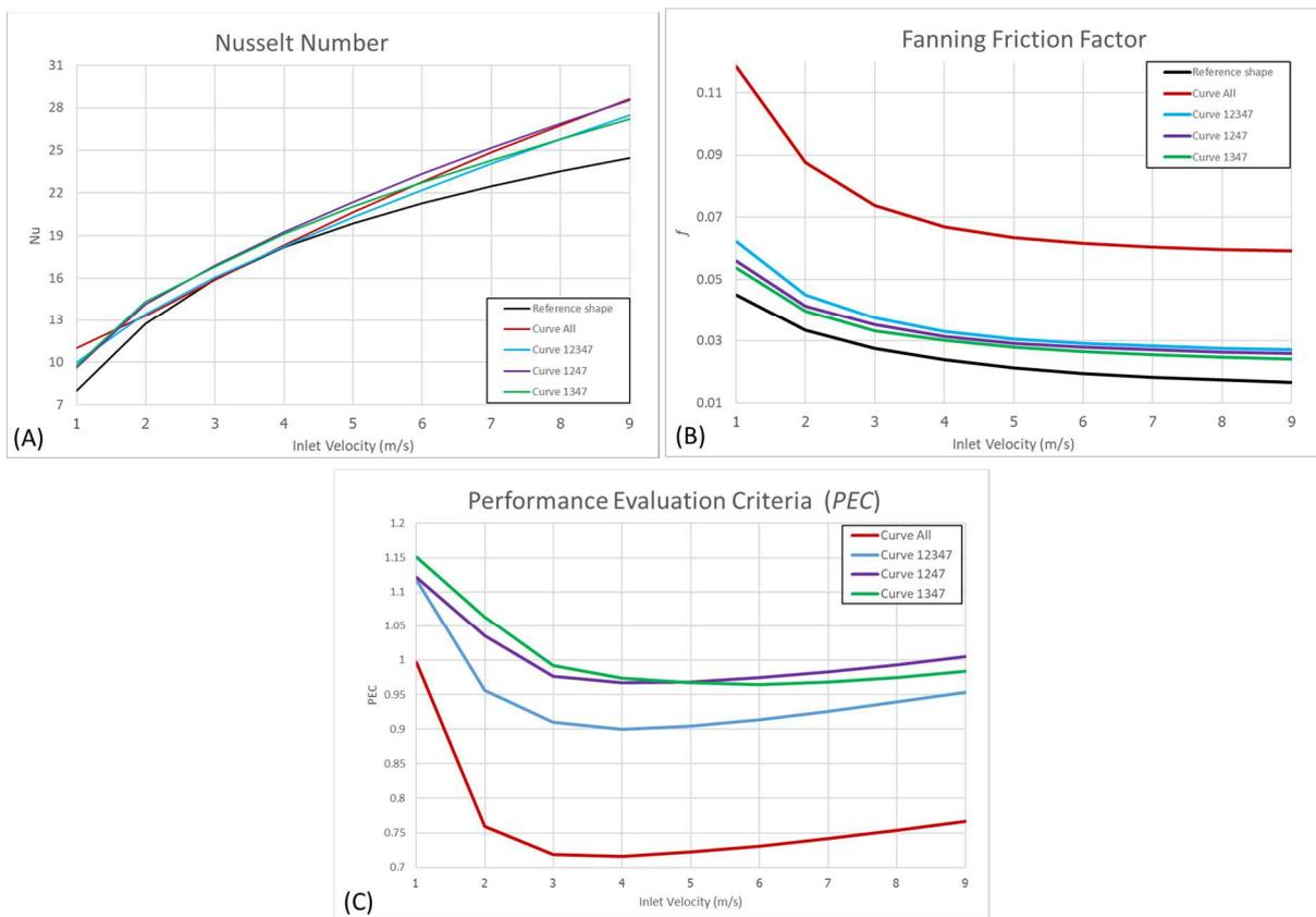
Fig. 10. Calculated results for (A) Nusselt number ( $Nu_h$ ) and (B) performance evaluation criteria (PEC).
