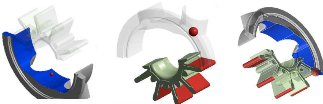
Fig. 5. Details on contact surfaces, between the deformable impeller (red) and the fixed pump body (blue).
