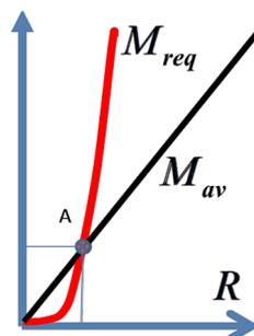
Fig. 4. The correlation of the required and available moments for aircraft control
