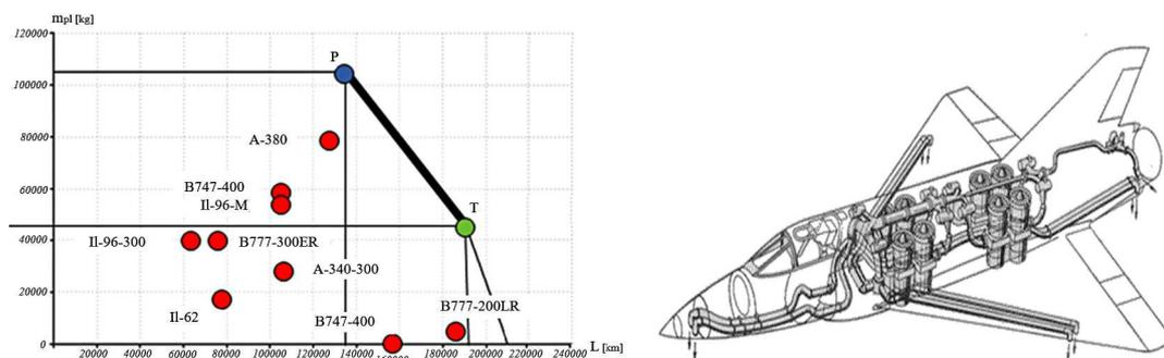
Fig. 1. Chart of payload mass – flight range depending on the takeoff weight of the aircraft
