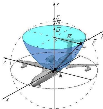
Fig. 3. Moment-inertial paraboloid of the aircraft
