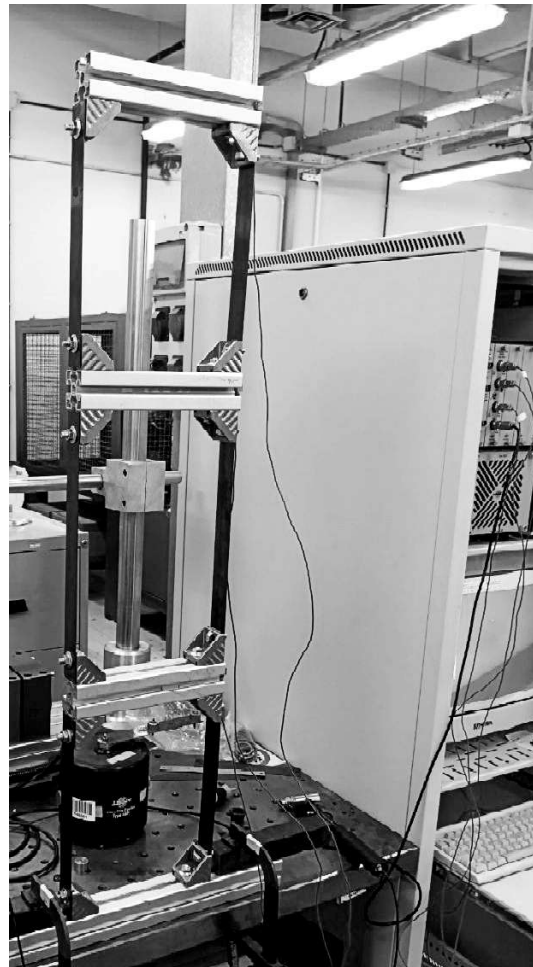
Fig. 26. Three-story frame structure analyzed in the experimental study.
