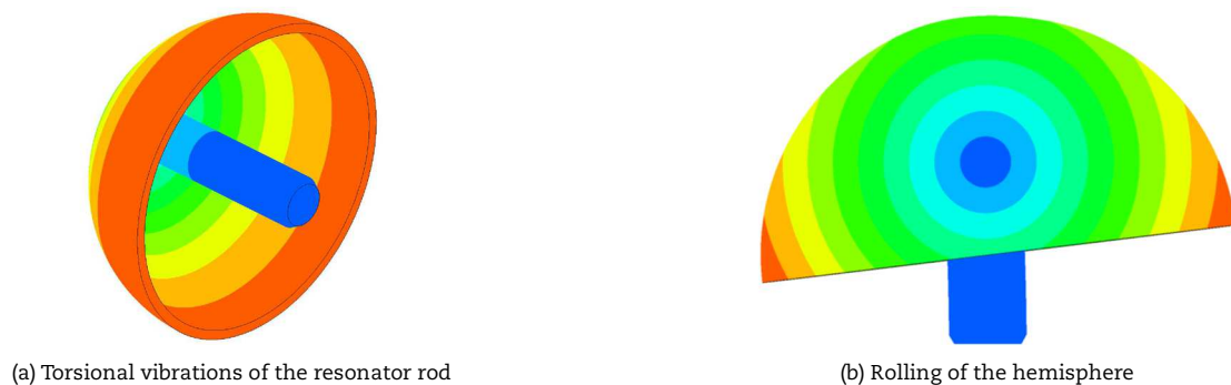
Fig. 3. Eigenforms of oscillations of the sensitive element of the RIG.
