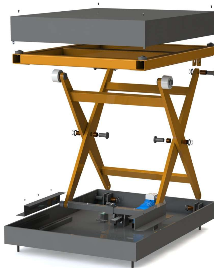
Fig. 1. CAD exploded view of the adaptive scissor lift mechanism representing the case study of this investigation.
