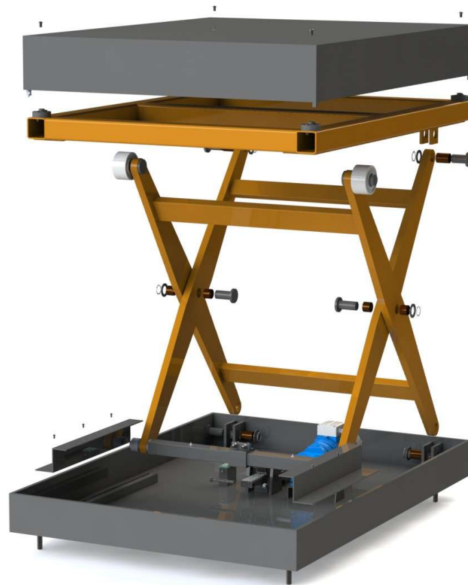
Fig. 1. CAD exploded view of the adaptive scissor lift mechanism representing the case study of this investigation.
