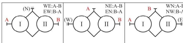
Fig. 6. Schematic overview of layout variant nomenclature according to cardinal points. The red letters A and B are used to denote the external shafts that are used to transfer power to or from the geartrain. The actual layout variant depends on the direction of the power flow being from A to B or from B to A.
