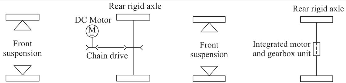
Fig. 2. Mechanical layout of a chain-driven (left) and of a compact drive (right) light electric vehicle.
