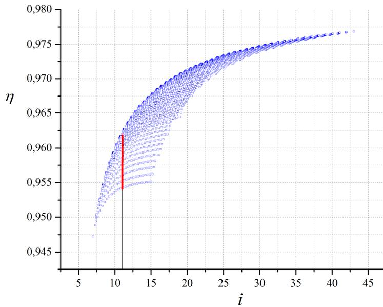
Fig. 7. Scatter chart showing the possible values of the efficiency ratio as a function of the overall transmission ratio  $i$  for the S16WN(E) PGT in the interval  $t_I = 1,5...6$  and  $t_{II} = 1,5...6$ .
