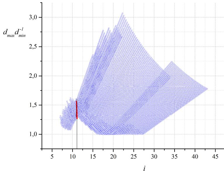
Fig. 8. Diagram of the ratio of the larger and smaller ring gear reference diameter as a function of the transmission ratio for the S16WN(E) PGT in the interval  $t_I = 1,5...5$  and  $t_{II} = 1,5...5$ .
