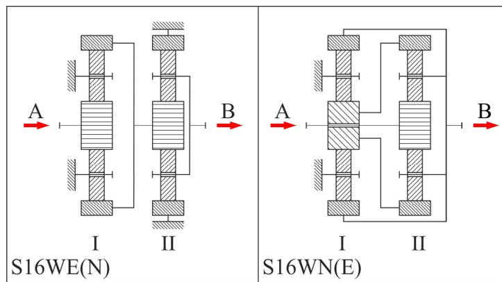
Fig. 13. Kinematic schemes of the S16WN(E) and S16WE(N) planetary gear trains.
