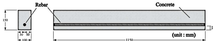
Fig. 3. Dimensions of the laboratory concrete beam specimen and rebar placement.
