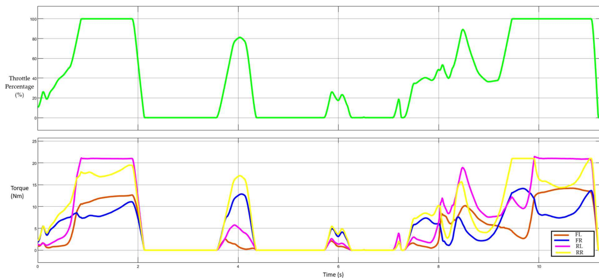
Fig. 16. Torque values for an open-loop configuration.
