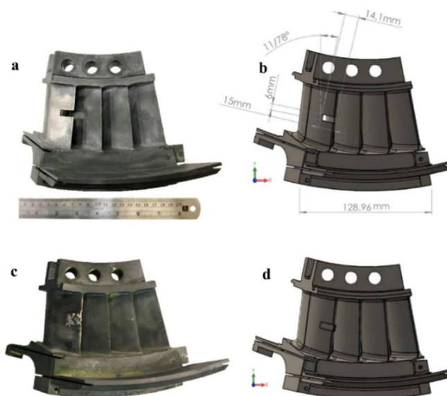
Fig. 1. (a,b) The removed cracked area at the trailing edge of the first vane of the gas turbine nozzle and its 3D CAD model; and (c,d) the repair welded gas turbine nozzle and the 3D CAD model for the assembled weld metal in the removed area of the gas turbine nozzle.
