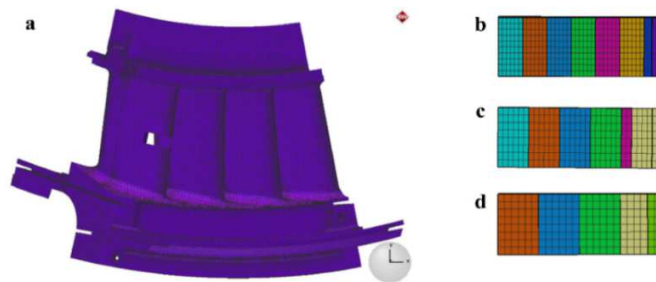
Fig. 2. (a) Mesh geometry of the gas turbine nozzle and (b-d) mesh geometry of the weld metal at different heat inputs: (b) 0.132 [kJ/mm], (c) 0.18 [kJ/mm], (d) 0.234 [kJ/mm].
