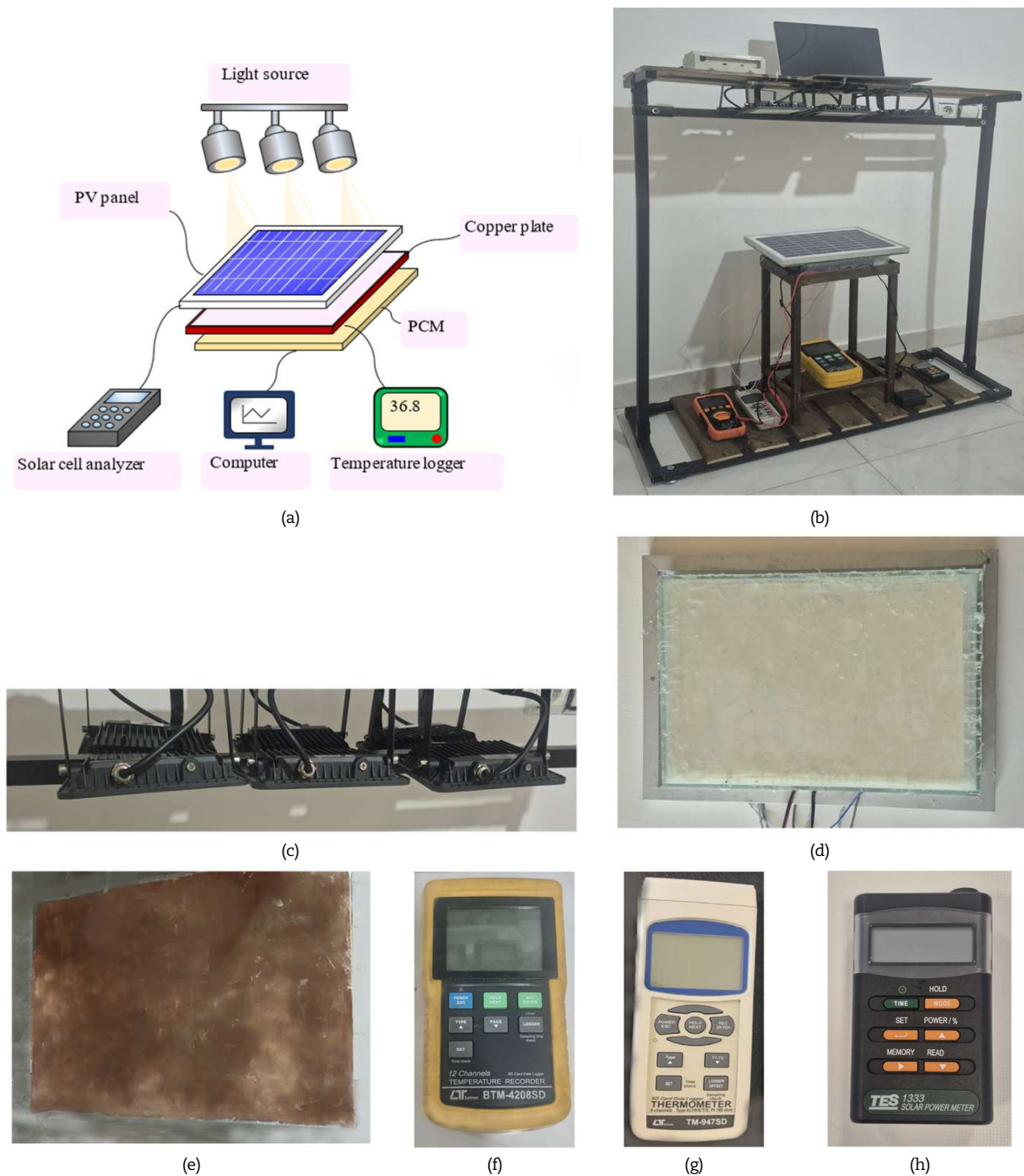
Fig. 18. Schematic representation and photograph of the experimental setup used to evaluate photovoltaic panel performance, (a) Schematic diagram of experimental setup, (b) Photo of experimental setup, (c) Lamps, (d) Integrated PV panel thermal storage container, (e) Copper plate, (f) 12-channel thermometer, (g) 4-channel thermometer, (h) Solar meter [74].
